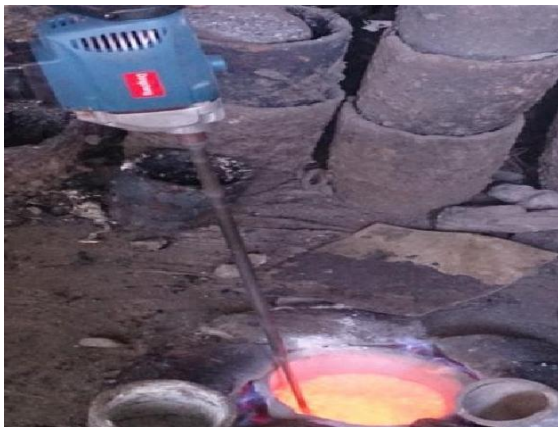
Fig. 1 stirring of Aluminium with Aluminium oxide
